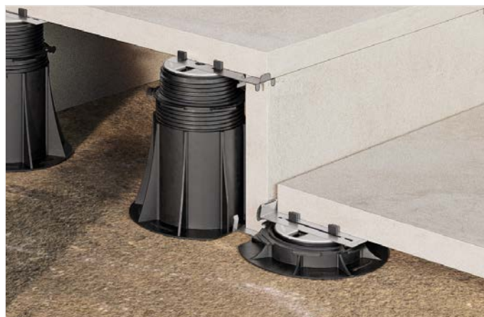
Installation of steps requires the vertical tile to be secured by a Head Clip and Base Clip on the pedestal.
